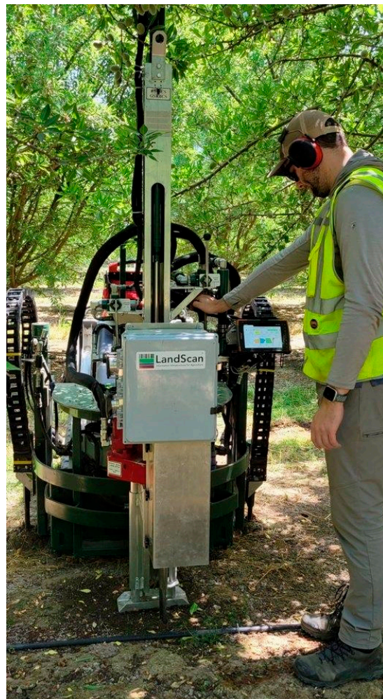
Figure 6. Digital Soil Core System, including the DSC probe, software, and deployment equipment.
